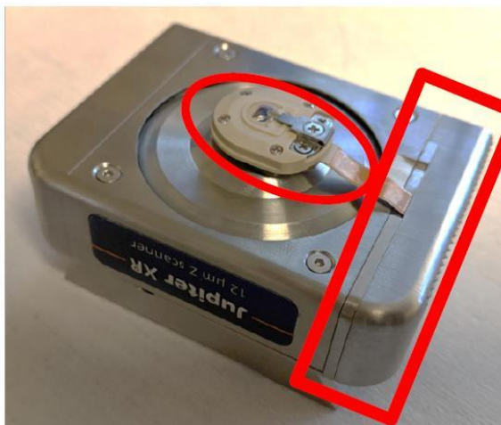
图 6-4 Z Scanner with Cantilever Holder
